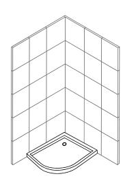
3, Fix the tray to adjusted position correctly and make sure tube to pipe well, avoid any water leakage!
