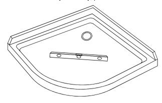
1, Check the tray by horizontal ruler, adjust the tray to correct level and keep stable!
